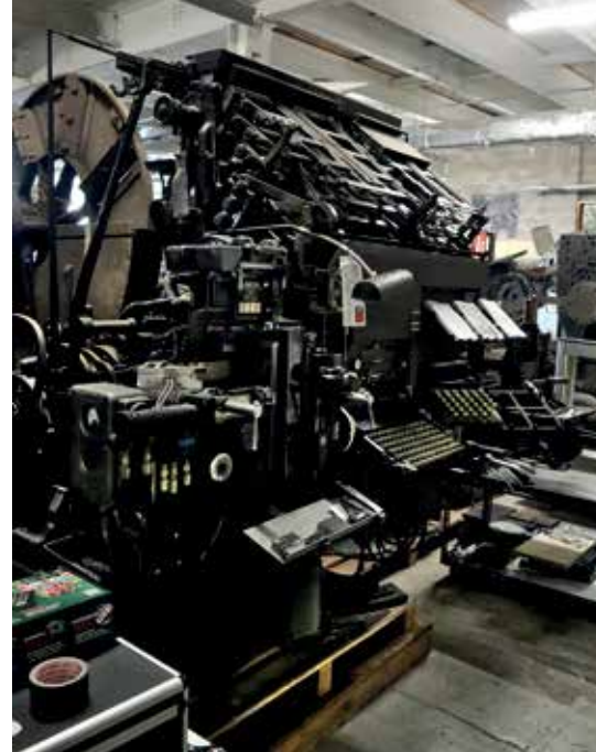
An old typesetting machine from a printer's in Kingswood – an absolute triumph of engineering genius and analogue complexity, long superseded by computers, and now in storage.
