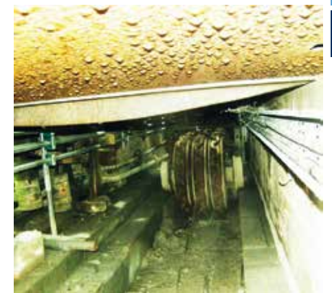
Under metal plates old hydraulic 'jiggers' which operated the lock gates can be found, an interesting early form of mechanization.
